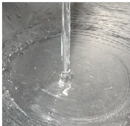
Fig. 6 Stagnation point flow: Liquid flowing onto a flat surface creates a situation of stagnation point flow, with shear forces increasing radially from the center point. Stagnation point flow can be found in vessel curvatures and branchings, i.e. the common carotid artery bifurcation into the internal and external carotid artery.
